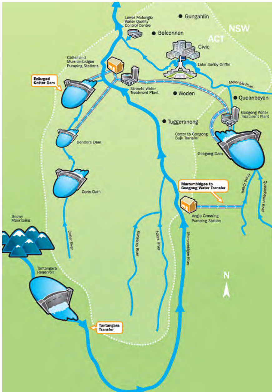
Figure 4: Key elements of the ACT and Queanbeyan’s water supply system (ACTEW, 2014)
