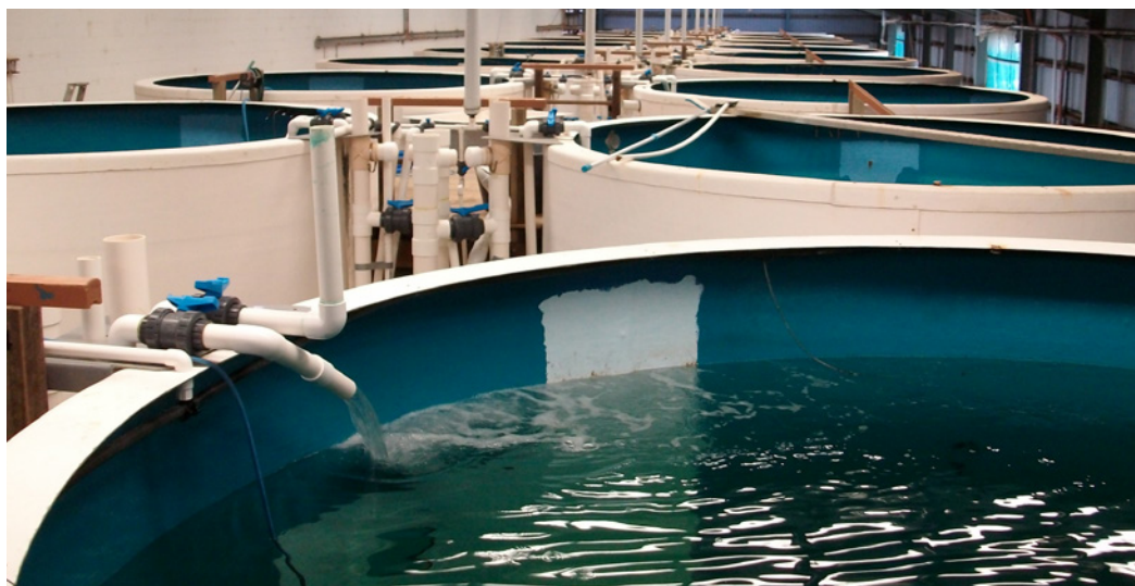
Recirculating tank system for barramundi ( Lates calcarifer )
