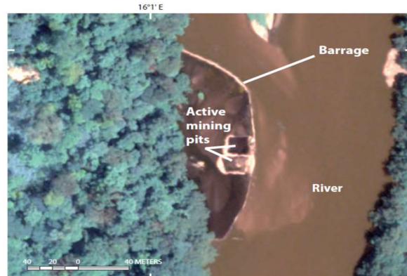
Figure 11. Example of a barrage built into a river channel to stem the flow of water to allow for the digging of pits. Satellite imagery of an area in the Berberati subprefecture of CAR from DigitalGlobe's WorldView-2 satellite, March 27, 2016.
