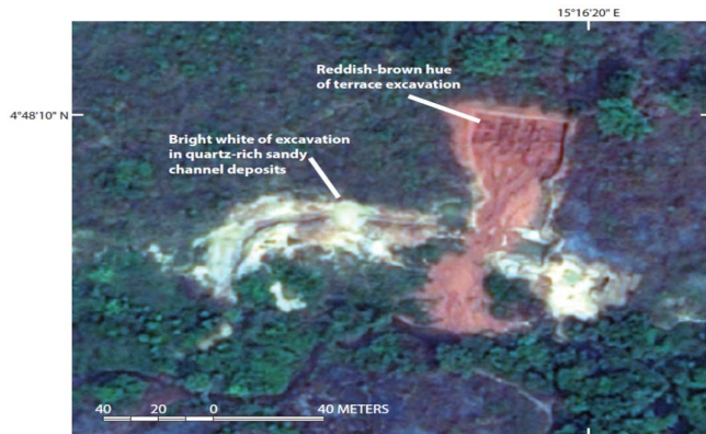
Figure 8. Photographic interpretation of artisanal and small-scale mining pits is partly based on tonal and hue differentiation, where bright white, tan, or red colors indicate excavation activity and are distinctive from the darker hues of undisturbed vegetated areas. Satellite imagery of an area in the Amada-Gaza subprefecture of CAR from DigitalGlobe's WorldView-2 satellite, February 21, 2016.
