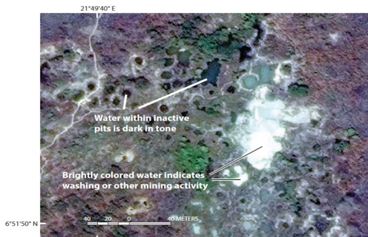
Figure 10. Pits may contain bright or dark-toned water, which can be used to indicate the recency of mining activity at that pit when supported by additional mining indicators. Satellite imagery of an area in the Bria subprefecture of CAR from DigitalGlobe's GeoEye-1 satellite, March 24, 2015.
