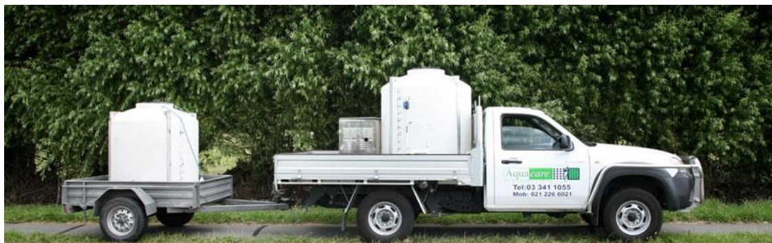
Figure 31 Example of sodium hypochlorite transportation
