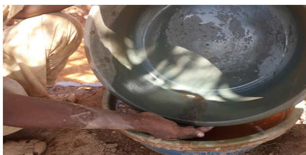
Figure 2.22: mercury amalgamation at Tilega, Zara area
