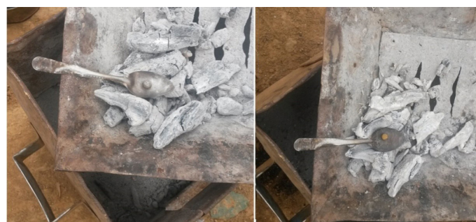
Figure 2.23: Burning of the amalgam to liberate mercury in open air using spoon; (a) Amalgam before heating (b) After mercury is evapo-rated (Kerksha area near Cosolda)
