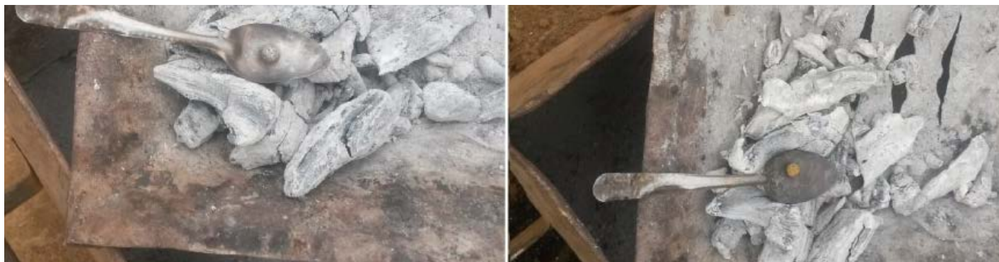
Figure 4. Open burning of the amalgam (Kerksha area near Kosolda); before mercury liberation (left) and after mercury liberation (right)
