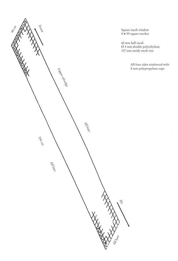
Figure 3: Inserting the window in the codend
