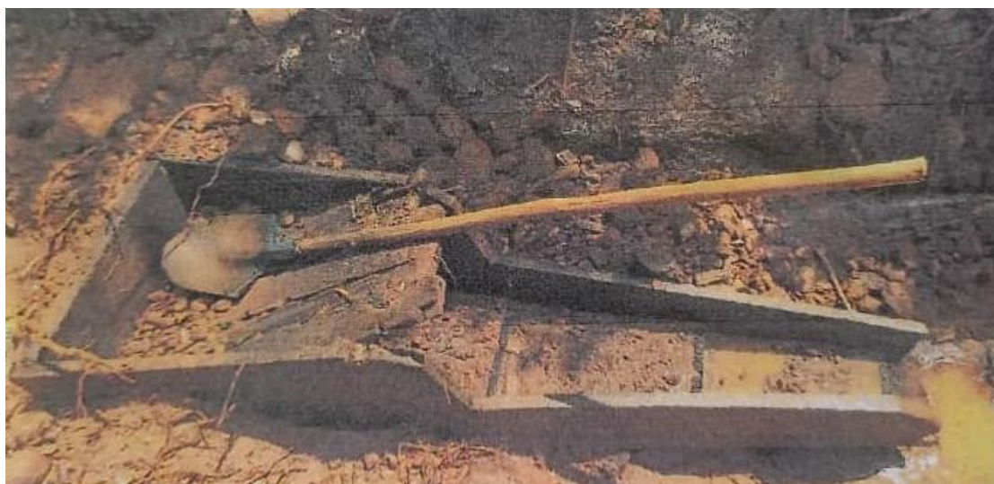
Figure 5 : Sluice gabonais (Camp 6 Mayibouth 2, Ogooué-Ivindo)
