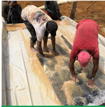
5) Mats are washed and beaten and materials concentrated. Mercury is then added
