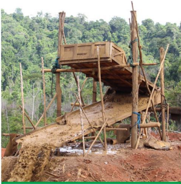
4) The slurry is loaded onto a sluice box (zig-zag) and the material moves downwards by gravity, where the material is separated into the lighter material and the heavier material which are associated with gold
