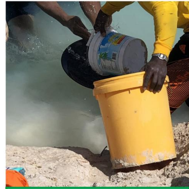
6) Concentrated material and mercury is decanted into a 5-gallon bucket, and final mercury amalgamation is done
