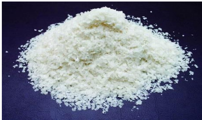
12 – Aka wood (Cellulose fibre powder ຫຼື wood fibre devised from wood pulp)
