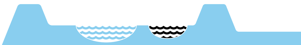
River widening - instead of dyke reinforcement
