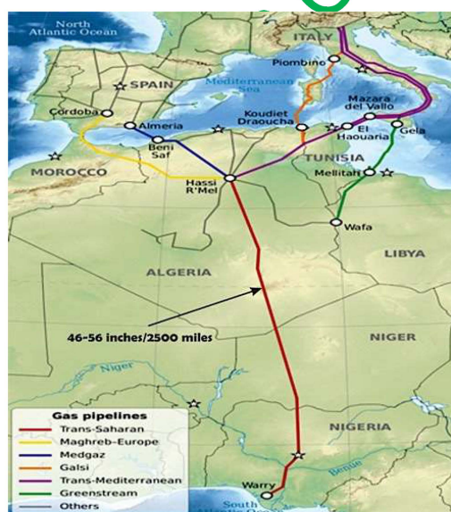
Figure 15: Trans-Saharan Gas Pipeline, Route
