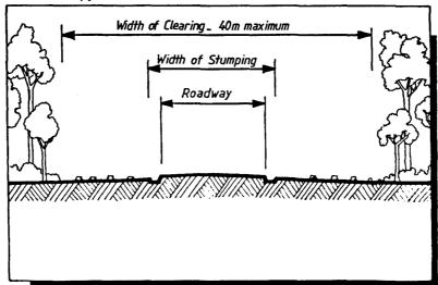
Typical Road Cross Section: Roadway and daylighting can almost always be accommodated within a maximum cleared edge to cleared edge width of 40 m. Excessive road clearance does not enhance drying from the sun.
