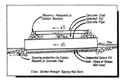
If pipes are used provide debris deflectors upstream and provide turbulence deflectors to assist fish passage, where this is required.
