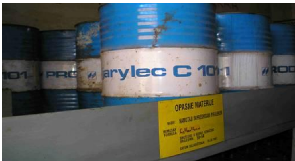
Figure 2.3.5.3.a: Stored equipment contaminated with PCB-based fluid
