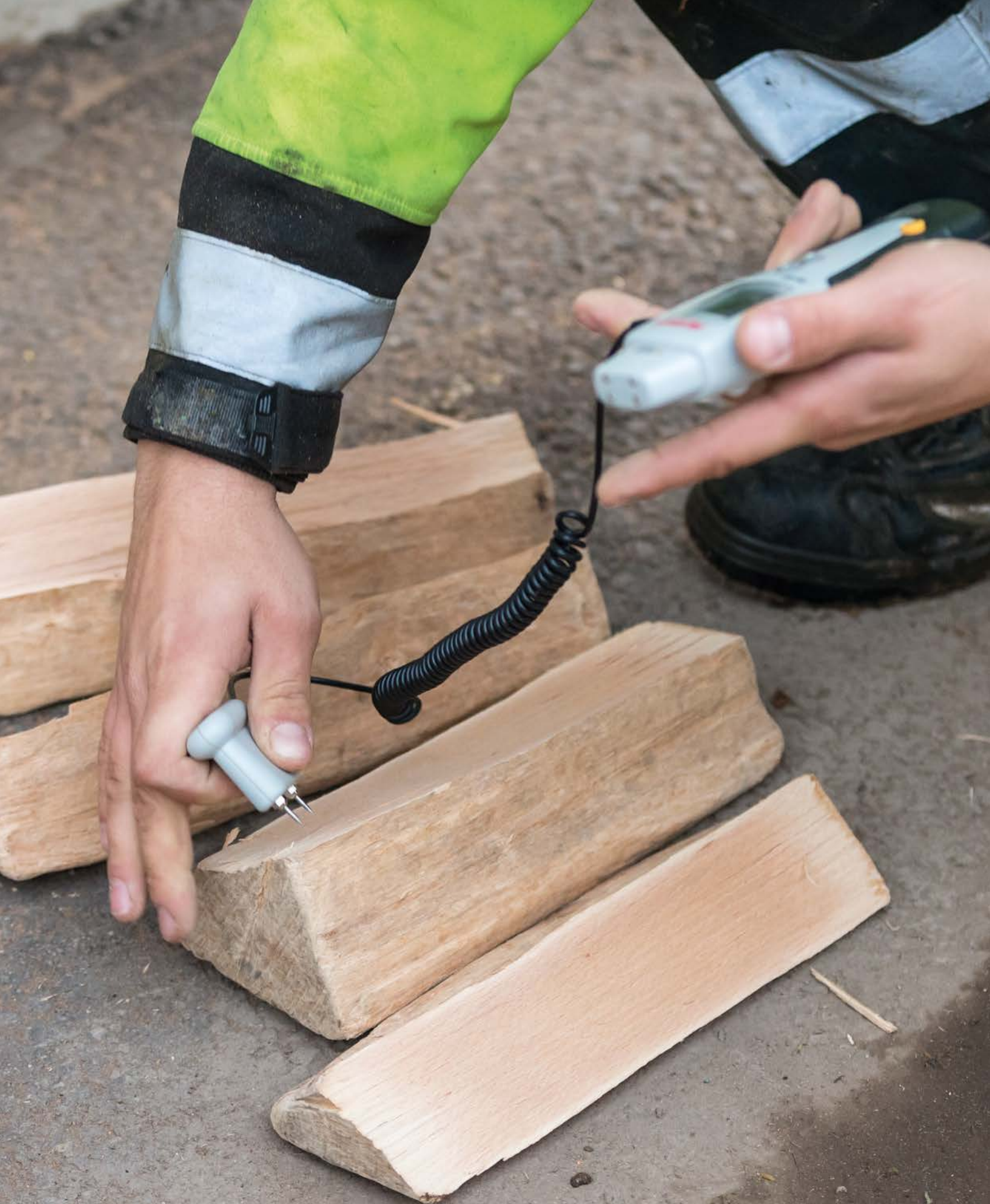
Measuring moisture in a beech log: the efficient and environmentally friendly use of energy wood contributes to fulfilling the Confederation's energy targets.
