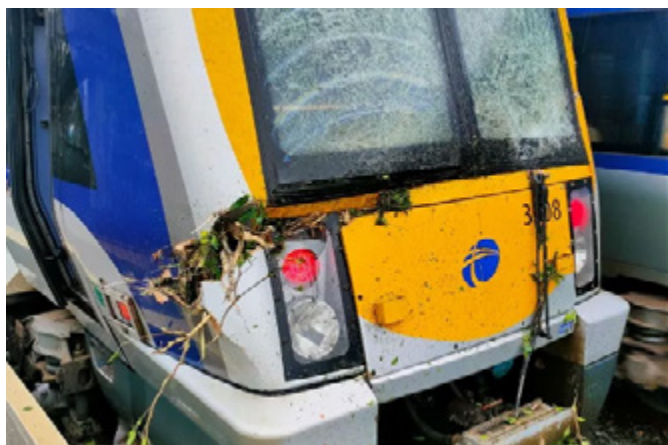
Image 4-5: Train damage from fallen trees (Translink)
