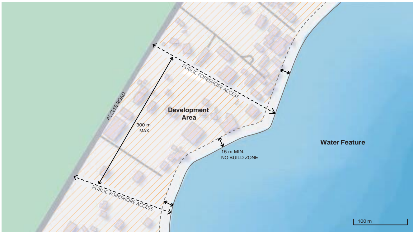
Figure 4: Diagram demonstrating required buffer between water features and new development and minimum provision for public access to foreshore.
