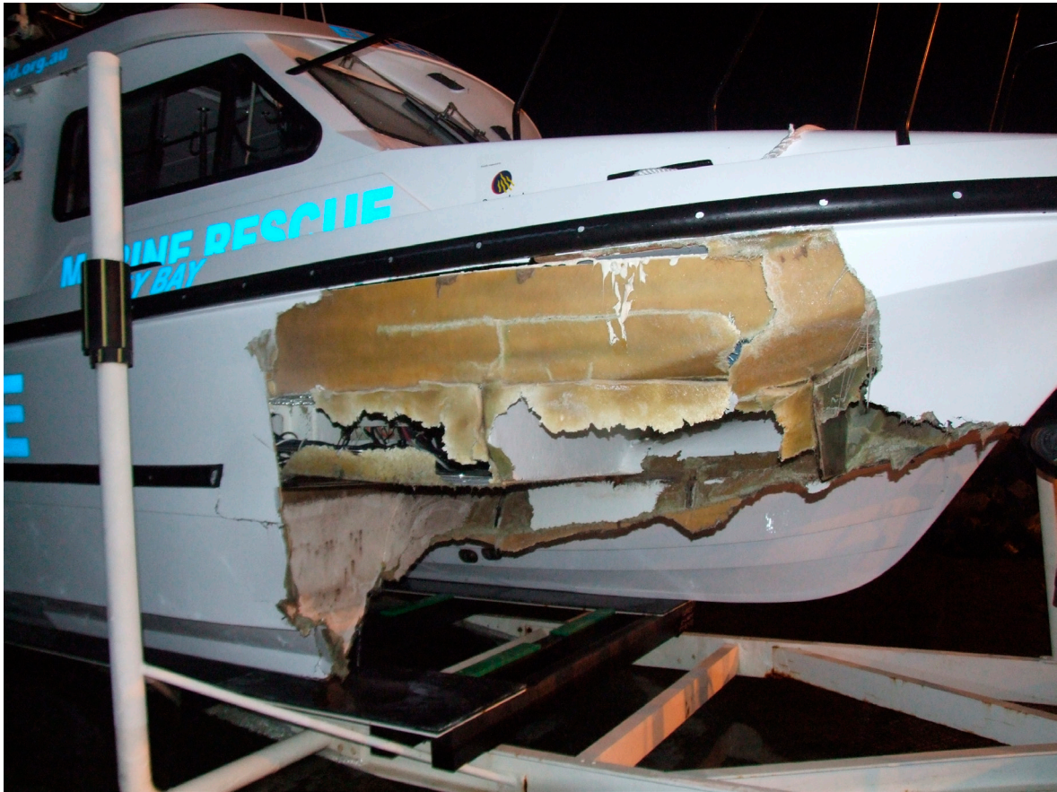
Photo: Marine rescue vessels may need to travel at speed during emergency operations. This image shows the damage to a marine rescue vessel following the collision with a whale © Copyright Marine Rescue QLD and Keith Williams.
