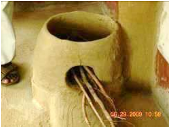
Figure 2.4: CSIR-IIR Improved Firewood Stove
