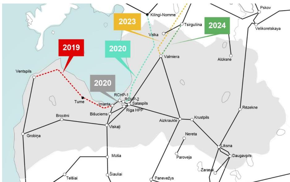
**Figure 40. The existing high voltage infrastructure network and planned projects<sup>152</sup>**
