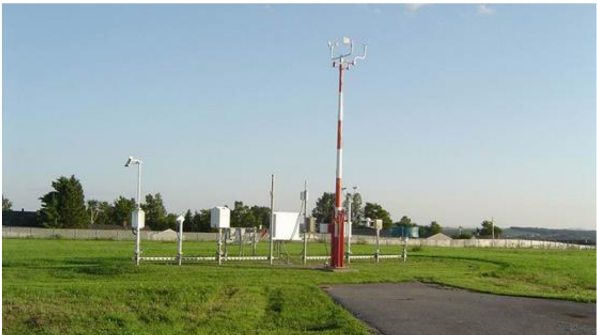
Figure III B 4 Typical weather station with wind tower
