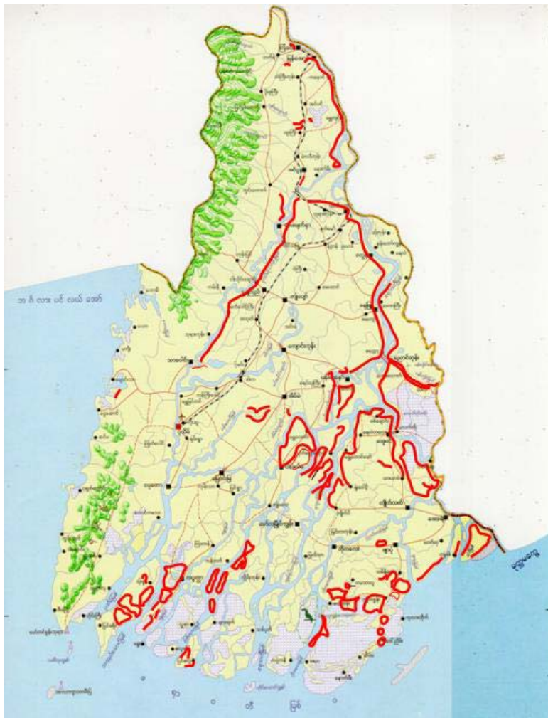
Figure A 24 Embankments (red lines) in Ayeyarwady Region [source MoAI, ID].
