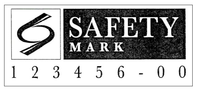
The complete Safety Mark comprises a safety logo enclosed in a square on the left, the words "SAFETY MARK" enclosed in a rectangle on the right and a unique 8-digit certification number traceable to the registrant running across the bottom of the square and rectangle. The colour is Pantone 287C Blue.
