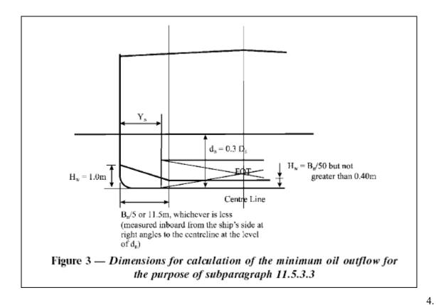
In the case of bottom damage, a portion from the outflow from an oil fuel tank may be captured by
